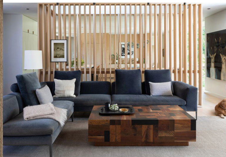
Partition wall made up of slats that rotate.
